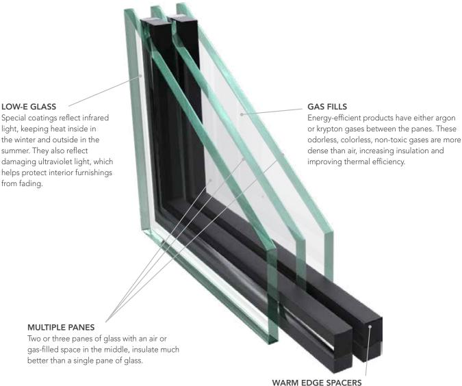
A spacer keeps the glass panes the correct distance apart. Non-metallic spacers insulate pane edges, reducing heat transfer through the window.
