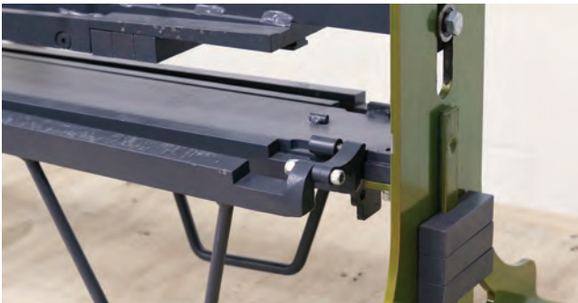
Fig. 23.3 - Shims in place (shim storage on the side)
