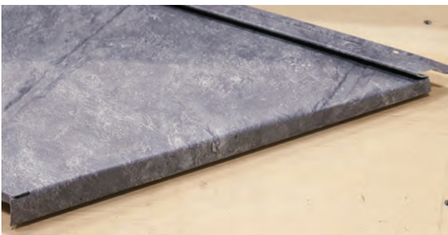
Fig. 25.4 - Finished tapered side lock
