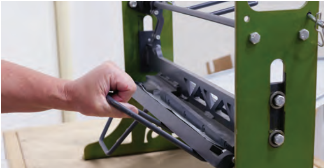
Fig. 25.2 - First side lock bend
