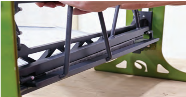
Fig. 25.3 - Final side lock bend
