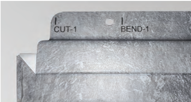
Fig. 19.1 - CUT and BEND marks on screw flange
