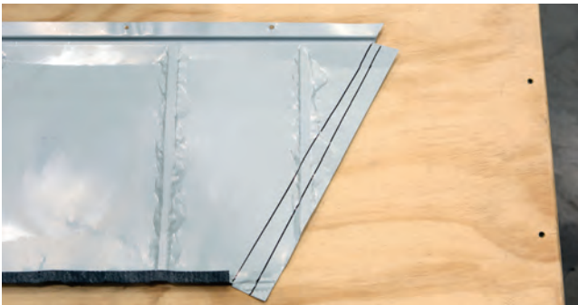
Fig. 21.3 - Panel marked and ready to fold
